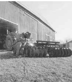
Harrow disk repair with Hobart 335A stick electrodes
