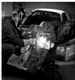
Automotive repair using the Millermatic 211 and HB-28 solid wire
